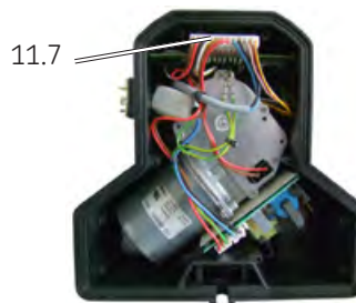
Plug of the control PCB Fig. 22
