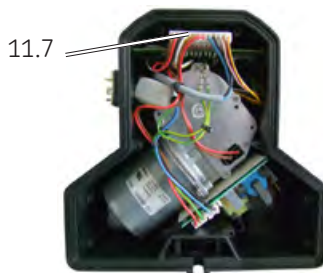
Plug of the control PCB Fig. 25
