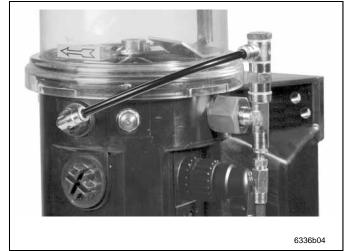
Pressure relief valve with grease return
