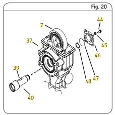
**46** Install the shaft cover (**46**) on the pump (**37**) (→ **fig. 20**).
