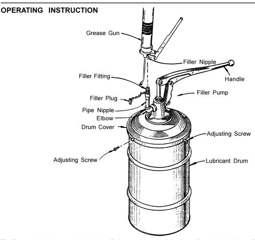
The filler pump is hand operated, designed to lift viscous and semi-solid lubricants from the original drums for loading the containers of the full range of Lincoln grease guns. These grease guns come equipped with a filler nipple for connecting to the outlet of the filler pump, which provides a quick and positive method of filling.
