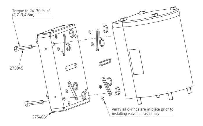
Notice Failure to torque the hex head capscrews (P/N 275045) to the specified torque may result in damage to your equipment and void the warranty of the product.
